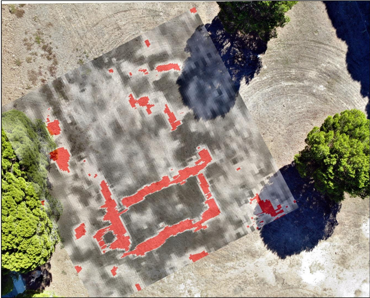
Figure 9: Gradiometer results showing location and orientation of subsurface anomalies, possibly the Church.
